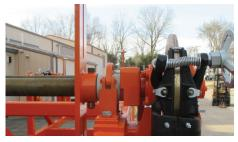
Quick change spindles lift straight out, requiring no tools. All wiring is protected by the frame and is engineered for optimum performance and safety.
