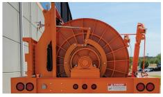
Spring applied, hydraulic pressure released safety brake is standard in the main drive line for operator safety. All unit operating controls are located at the operator's station, off the ground, for operator safety.
