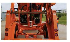
Levelwinding is simplified by allowing the operator to accurately guide the rope or conductor during pull-in or payout operations. The V-groove permits easy handling of cable splicing sleeves and accommodates a wide variety of cable, rope or conductor diameters. Replaceable segments assure quick replacement of bullwheel lining should hard usage cause excessive wear.
