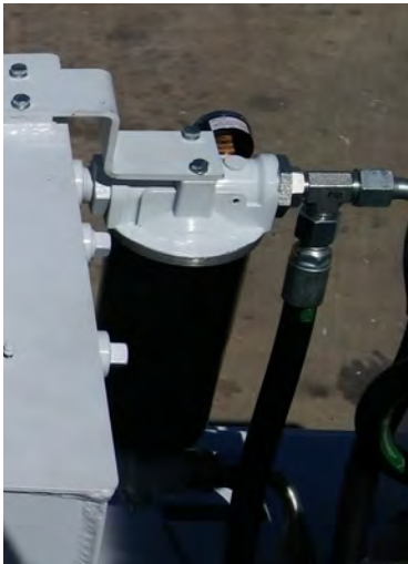
Figure 16: Hydraulic Fluid Filter
