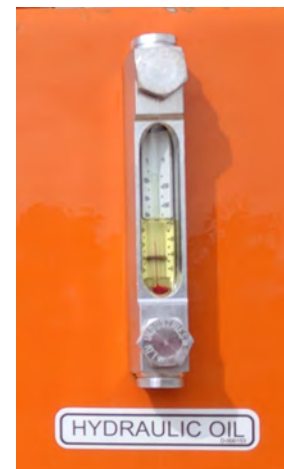
Figure 5: Hydraulic Oil Level Gauge w/ Temperature Indicator
