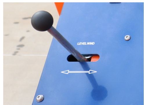
Figure 8: Levelwind Horizontal Control
