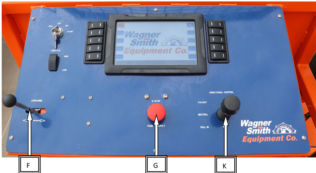
Figure 10 (repeated): Control Panel
