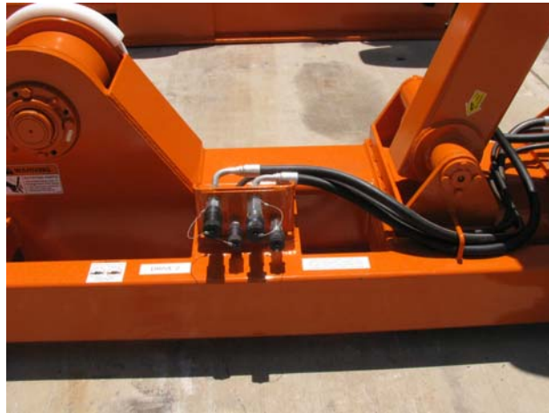
G. Drive 2 bulkhead bracket, contains quick disconnect fittings for Drive 2.
