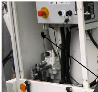
The boom control lever hydraulically adjusts the height of the boom.
