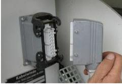
Insert remote control cable plug into connection.
