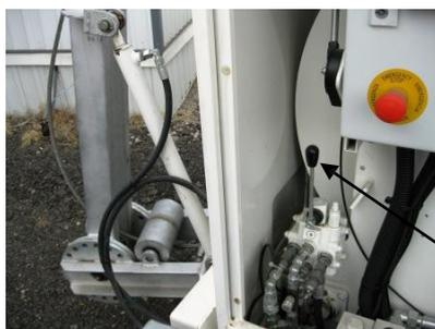
**Pos. 18 Hydraulic control lever to raise and lower boom**
