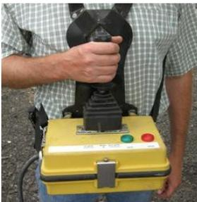
To pay-out the wire rope, push the lever right while holding down the dead-man switch on top of the lever. For pulling-in, move lever left while holding down the dead-man switch. The amount you move the lever increases or decreases the line speed.
