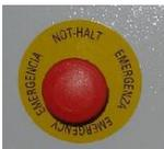
When the emergency stop button is pressed, the winching function will be stopped immediately. Reset by turning left.
