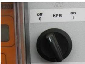
For monitoring the winching process with the KPR 2000, set the switch to ON
