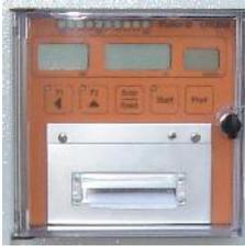
**Pos. 9 Electronic Measuring System (KPR 2000)**
