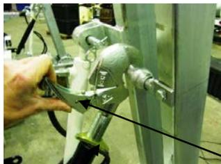
Latch used to disconnect ball coupler from boom when hydraulically lowering boom. Reverse procedure to secure boom for transport.
