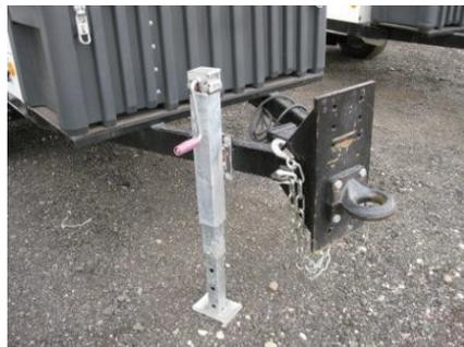
**The hitch can be adjusted in the range of 2.165 inches (55 mm) steps.**
