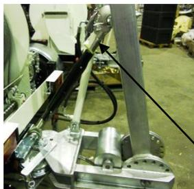
Adjustable boom lock is used to secure the boom when unit is being transported. The boom lock must be secured when transporting to prevent boom damage.
